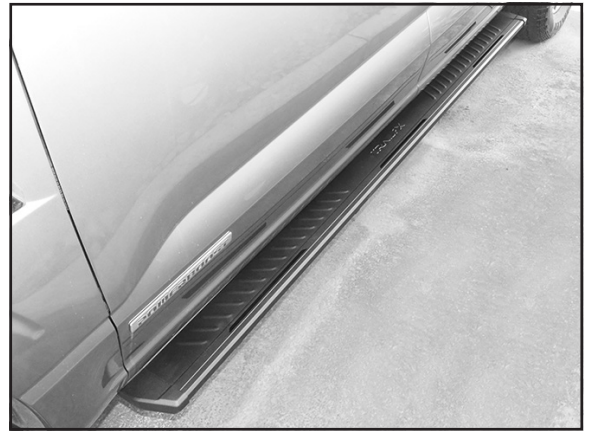
(Figure 14) Complete driver/left Running Board installation.
